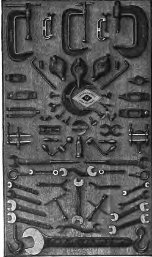
Fig. 170. Typical Drop Forge Tools Courtesy of J. H. Williams and Company, Brooklyn, New York
